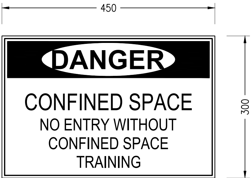
CONFINED SPACE SIGN DETAIL SCALE 1:20
